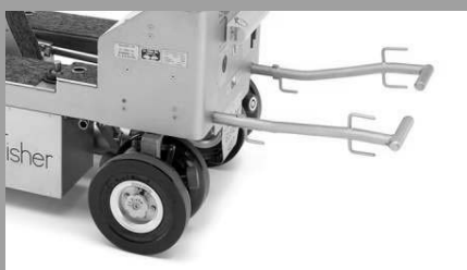
PUSH POSTS DOUBLE AS REAR CARRY HANDLES
